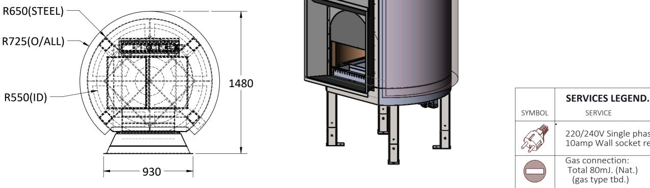
OVERALL DIMENSION INCLUDES 50mm INSULATION +25mm AIR GAP
